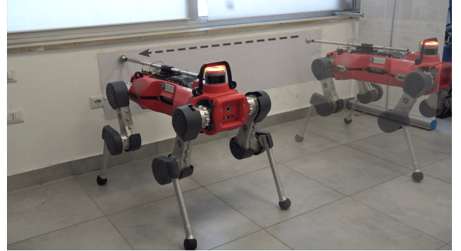
Fig. 1. A quadruped robot performing a push-and-slide task using a stick rigidly attached to its base. The transparent robot indicates the starting pose; the opaque one indicates the final pose. The dotted arrow denotes the sliding path of the end-effector on the wall.
